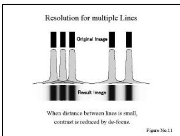
Since Tripitaka Beijing Edition is a character-base text, resolution of multiple lines are the most important. By the de-focus effect, the gaps between two lines are getting dark. Thus, the contrast among lines is reduced in proportion to the line distance.
