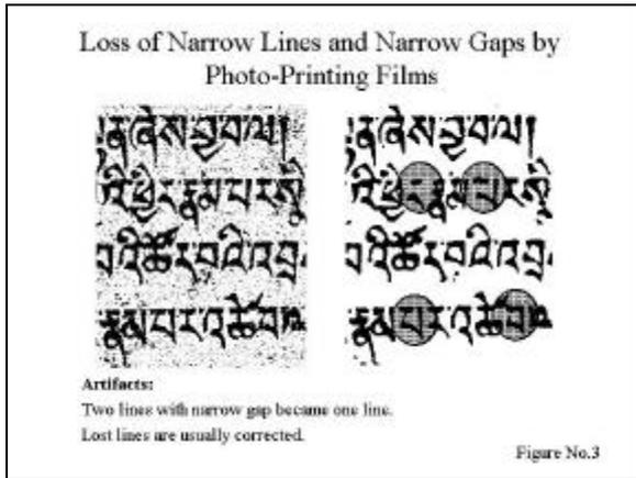
Here is the example of Photo-Printing quality. The left figure is taken by a good scanner, and the right figure is a simulation of photo-printing.
