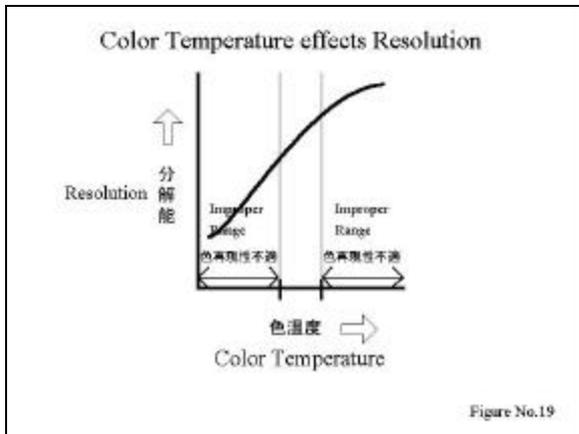
For the fidelity of colors on the original, the color temperature should be set at 5,500 degree K.
