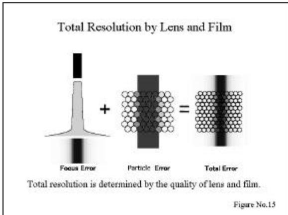
As the result, total resolution is determined by the quality of lens and film.
