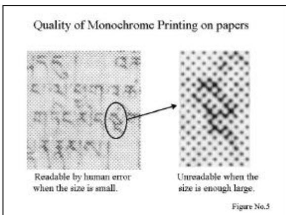
Half tone monochrome printing uses different size of dots to show half tone. In this case, multiple dots show one small region. Thus, resolution of half tone monochrome printing is lower than the value of resolution. This means half tone monochrome printing on papers contains large quantum noise.
