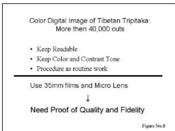
Since the size and amount of Tripitaka Beijing Edition are too large, 35mm reversal color film with micro lens was selected. 35mm camera is easy to use and cost of 35mm film is not large. For more than 40,000 cuts, conditions for the routine work should be determined. Thus, quality proof for above condition was researched.
