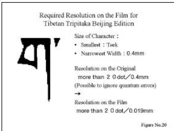
Based on our research, at least 20 dots for 0.4mm on the original was required to ignore quantum errors. Of course, this dot density is specific to the original.
