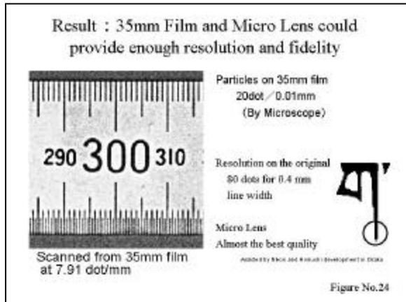
This slide shows our result that is a scanned data of the photo of certified metal scale from 1.3m distance. 0.15mm width lines with 0.5mm distance can be clearly separated.
