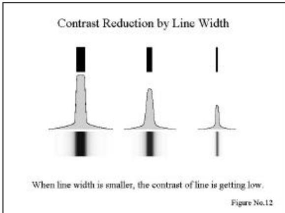
By the aberration of a lens, the contrast of narrower line is getting low. And the reflection from crystals on a film reduces the contrast of narrower lines.
