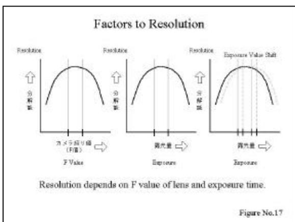
The aberration of a lens can be reduced by larger F value. But if the diameter of aperture is too small, the resolution is getting worse by the diffraction effect of diaphragm.
