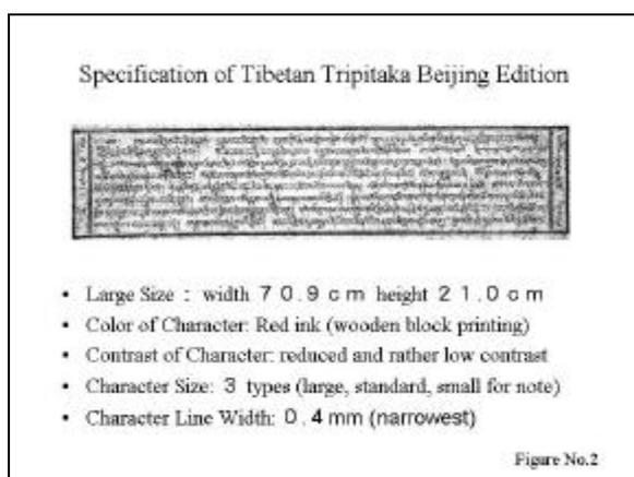
Before starting making digital image data, characterizing the original is essential. As we know, digital image is created by collection of small dots called pixel. The size of pixel must be enough smaller than the smallest line on the original. If the size of pixel is not enough smaller, quantum noise strikingly reduced readability. Also the overall size of the original can be used to determine the process and procedure of digitizing.
