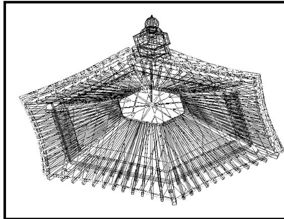
(9b) Roof - wire frame 3D CAD model
